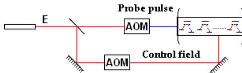
Figure 6: Experimental setup for the storage of a probe pulse
