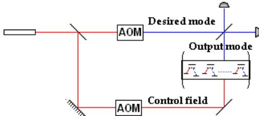
Figure 7: Experimental setup for the retrieval of a probe pulse
